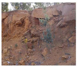
Typical Darling Range cross section showing surface caprock with underlying pisolite material
