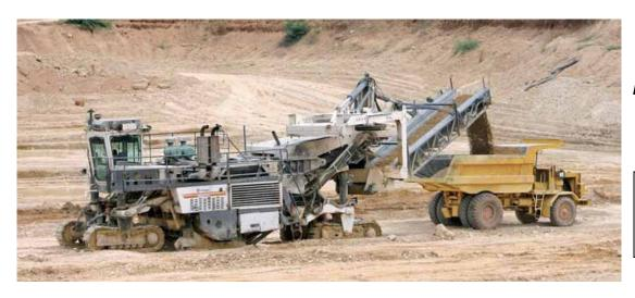
Continuous Surface Bauxite Mining; strips, crushes and loads in one process.
